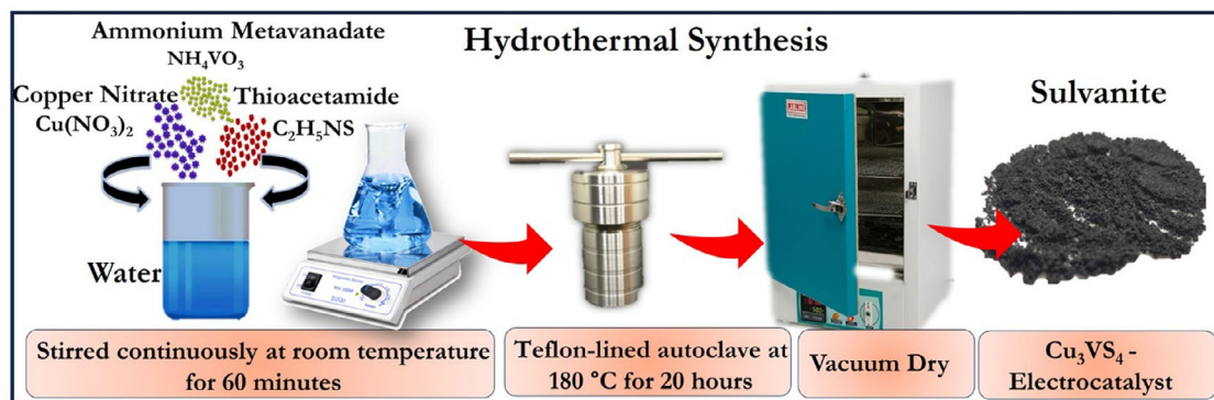
SCHEME 1 | Schematic of the synthesis procedure of the ternary chalcogenide (CVS).
